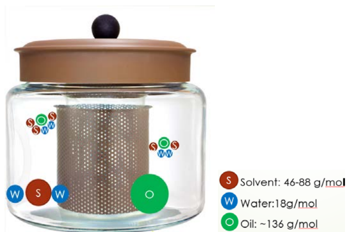
Figure 1. OilExTech's EssenEx™ 100 unit consists of a 2 L glass jar, a 250 mL beaker surrounded by Teflon coated mesh, and a 200 mL ice core. The oils are condensed on the ice core and collected in the beaker. The collection beaker is then poured into a volumetric flask, where the oils are separated from the water. Solvent, oil, and water molecules are included to demonstrate how oil is carried to the ice core.
